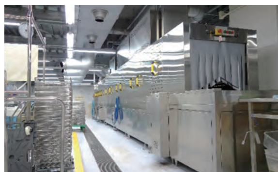
飼育ケージ洗浄装置 (Tunnel washer for housing cages)
