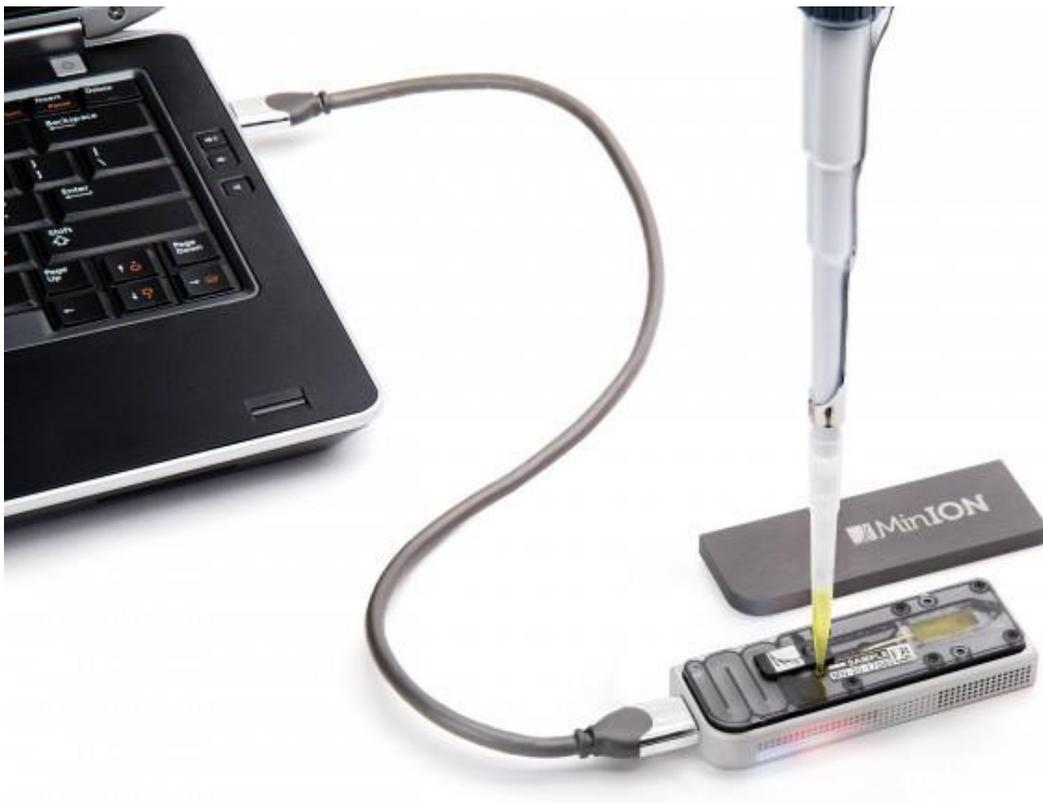
DNA can be sequenced by threading it through a microscopic pore in a membrane. Bases are identified by the way they affect ions flowing through the pore from one side of the membrane to the other.
