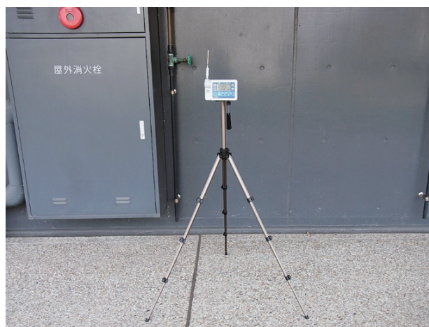
Figure 2 Air sampling at the new building of the National Institute of Health Sciences Left: Trace volatile organic compounds analysis room, E-17; Right: Outdoor
