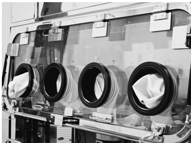
Fig. 1. An image of the Sterility Test Isolator 3 D Clean System installed in National Institute of Health Sciences
