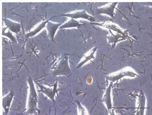
Fig. 2 Phase contrast micrograph of fibers of CMBA precipitated in the culture medium after its DMSO solution was added. Single and bundled fibers are shown ranging the length from around 2 to 33 \mu\text{m} . Bar indicates 50 \mu\text{m} .
