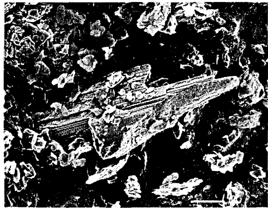
Fig. 3-b. Multi-layered slate-like appearance of tremolite. Bar: 10 \mu m
