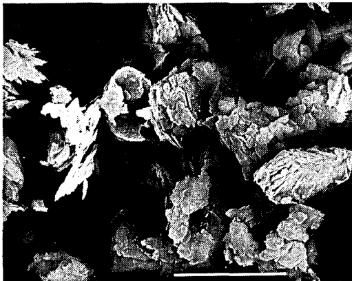
Fig. 1-b. Higher power view of talc crystal clusters. The surfaces are petal-like. Bar: 10 \mu m
