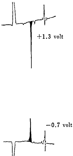
Fig. 5 HPLC of Aflatoxin B 1 with voltammetry HPLC conditions: Column 0.4 mmφ×250 mm, Yanapak ODS-T, Mobile phase CH 3 CN-acetate buffer (pH 4.0) 52:48
