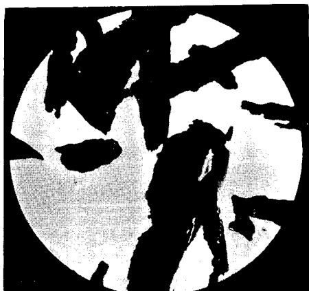
Fig. 4. Alloy particle of coarse cut \times 185
