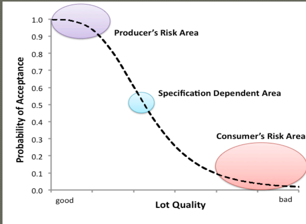
図 2. A typical OC curve showing test characteristics
