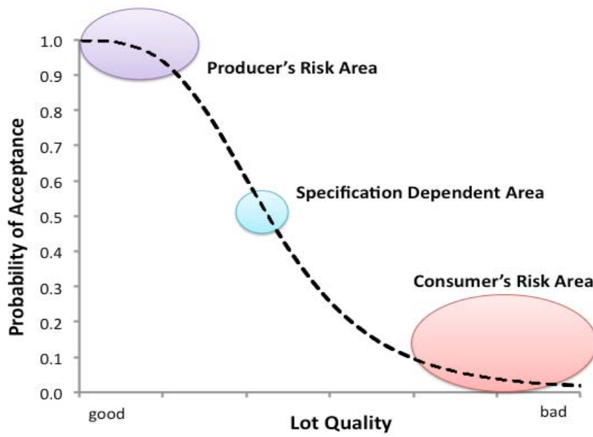
図 2. A typical OC curve showing test characteristics
