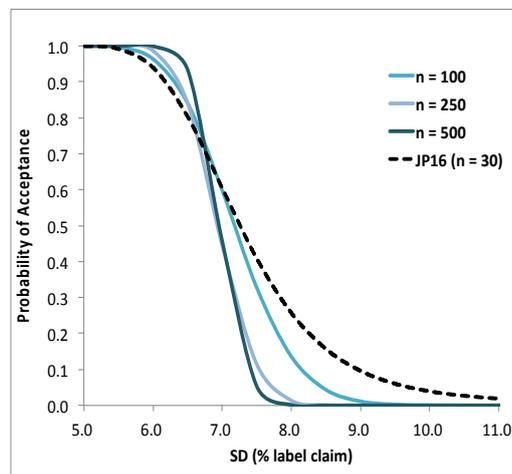
図 3 OC curves of UDU tests recommended by PhRMA
