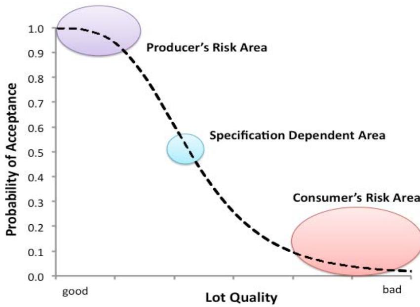
図 2. A typical OC curve showing test characteristics
