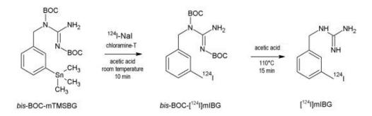
FIG. III-8. Synthesis Route for Preparation of [<sup>124</sup>I] MIBG
