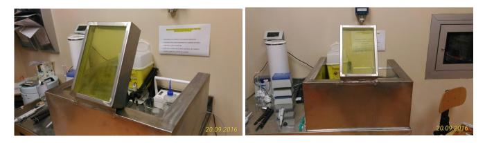
FIG. 5. Example of an inexpensive lead-shielded area for the manipulation of QC samples.
