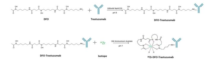
FIG. III-5. Steps Involved in the Preparation of [<sup>89</sup>Zr] DFO-Trastuzumab
