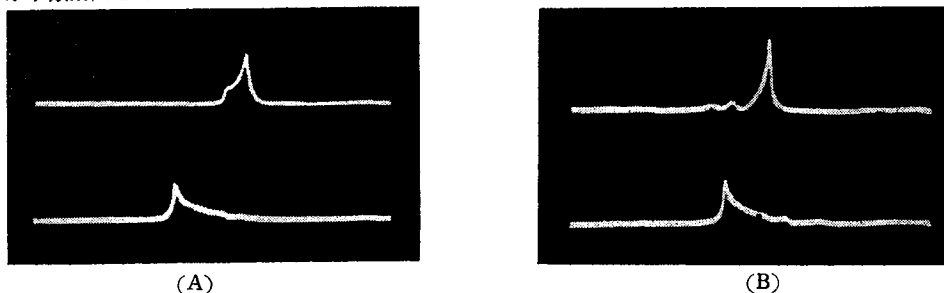
Fig. 1. Ascending and Descending Electrophoresis Patterns of Cryst. BA and Cryst. BB, (in 0.18 ionic strength hydrochloric acid-potassium chloride buffer of pH 2.2.)
